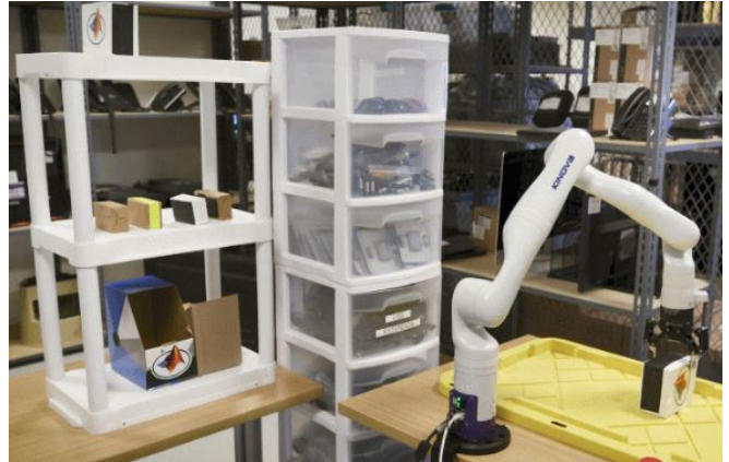
Fig. 1. The experimental setup where a Kinova ® Gen3 robotic arm performs a pick-and-place task in a warehouse environment. The Robotics System Toolbox ™ [12] Support Package for Manipulators is used to interface with and control the robot arm using MATLAB ® [9]. Stateflow ® [13] for MATLAB ® is used to schedule the pick-and-place tasks. The corresponding simulation environment is shown in Fig. 6. A video of the experiment results is provided in https://github.com/stacymav/nonlinearmpc-content .
