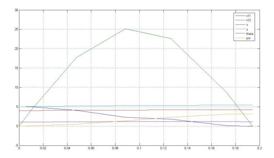
After applying Claim 2A, the system is supposed to go from a sticking mode to slipping mode where steering angle velocity becomes zero. We can observe exactly same dynamics in the figure given above. Here, variable v12 represents the steering angle velocity. After increasing for some period, it decreases to zero and system goes into slipping mode.
