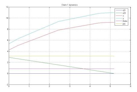
As we know, system should come to a complete halt after it has been controlled by claim 1. If we have a look at the graph, we can see that all the variables representing the position of the Roller racer (x, y, theta, psi) are stabilized after finite time i.e. System is now in the rest mode. Similar results for some different initial configuration of the Roller racer are shown below.
