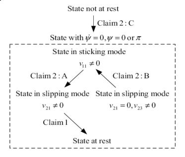
As stated earlier, there are three modes of operation of the Roller racer namely Sticking mode, Slipping mode, and Rest mode. The conditions required to be satisfied for the Roller racer to be in any particular mode are shown above in the figure. In addition to that, different claims which can be used to jump between each of those modes as and when required. When the system voids any particular constraint to
