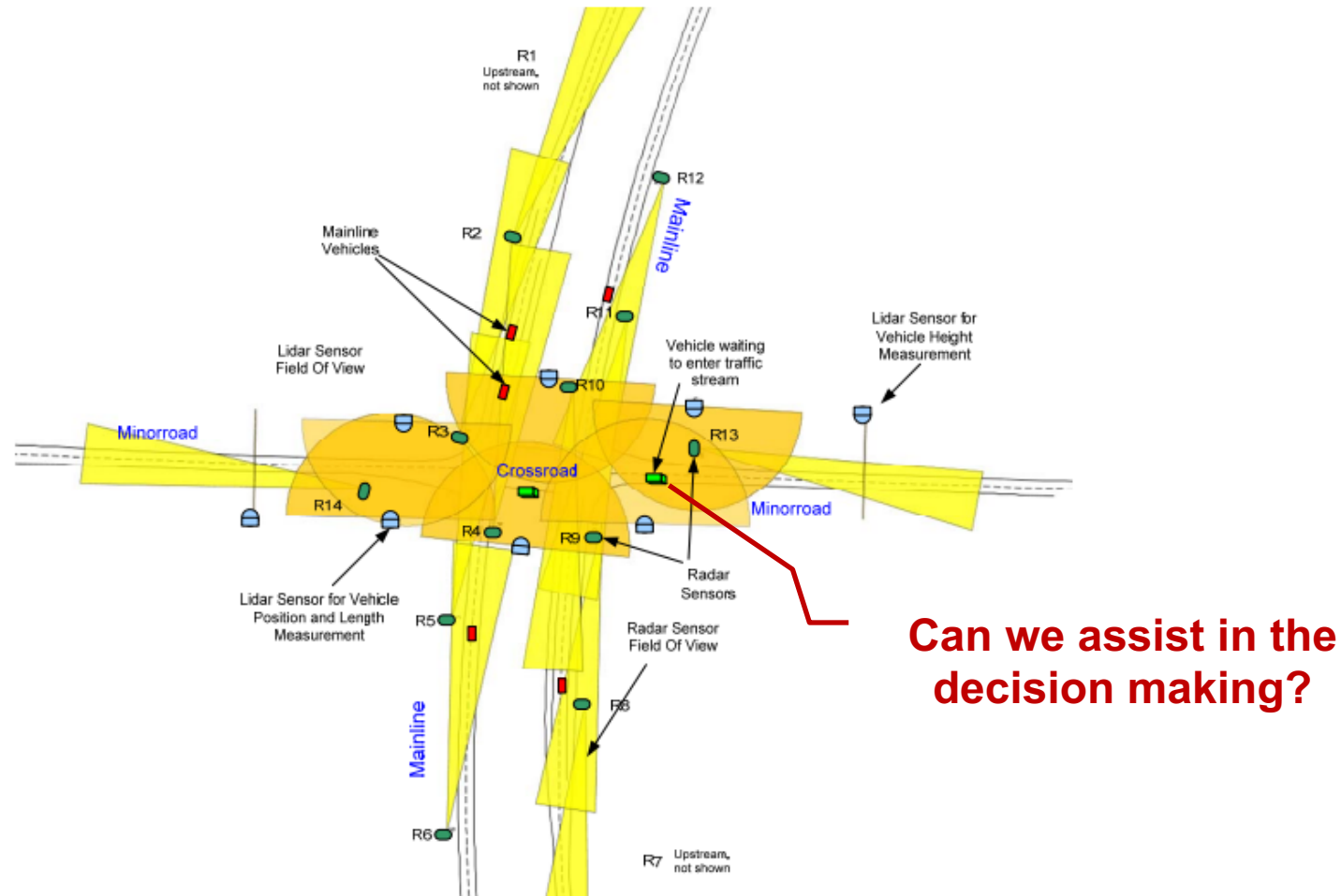
Figure 1: Plan view of a typical instrumented rural four lane expressway intersection. Sensors are radar (yellow triangles indicate field of view and) scanning lidar (orange semicircles); all data is sent from sensor processors to the main central processor.
